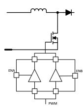
Figure 12. A large switch driver by two paralleled outputs with minimized mismatch (IVCR2403/4)
