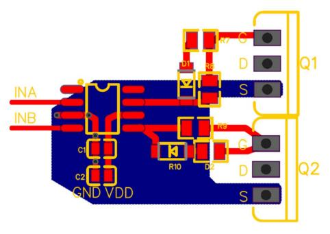
Figure 13. Layout Example for IVCR2403/4/5
