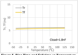
Figure 5. Rise Time and Fall time vs Temperature
