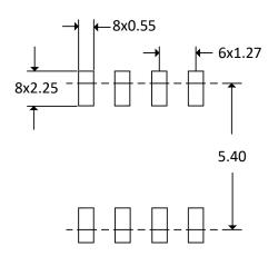
SOIC-8 Recommended Soldering Dimensions
