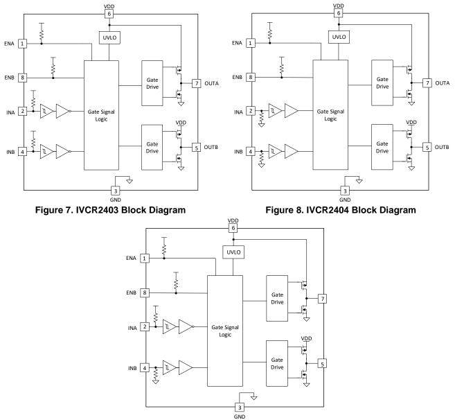
Figure 9. IVCR2405 Block Diagram
