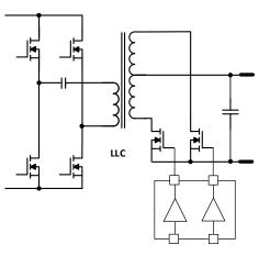
Figure 10. Two channels driven separately (IVCR2403/4/5)
