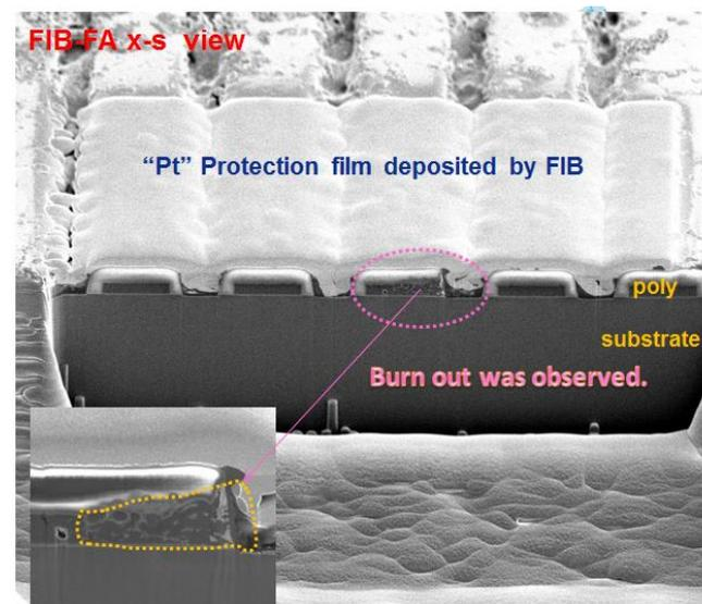
Fig.10. SiC MOSFET defect root cause found
