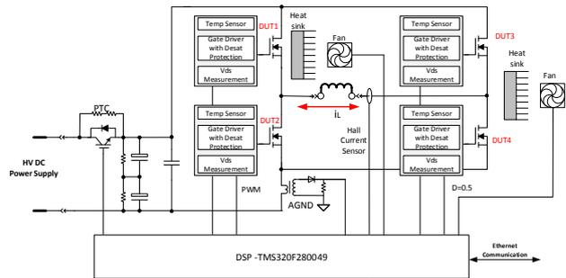
Fig. 2. Hammer and burn-in system diagram
