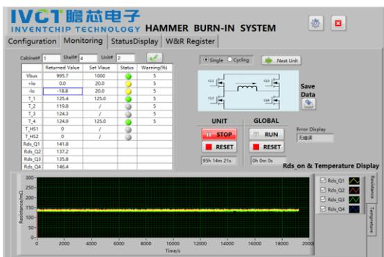
Fig. 8. System monitoring window
