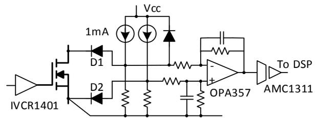
Fig. 5. High-speed isolated Vds sensing circuit
